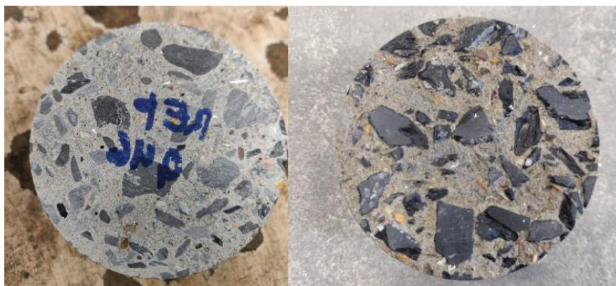
Figure 5.15 - Surface of a concrete specimen (REF0.46) before (left) and after (right) 28 freeze-thaw cycles with de-icing salts (3% NaCl solution).
