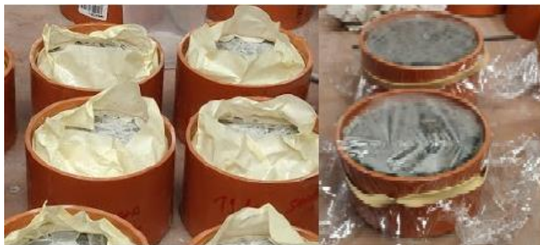
Figure 5.17 - Preparation of specimens for the freeze-thaw cycles. The molds filled with epoxy are shown on the left and the sealed specimens after receiving the saline solution on the right.
