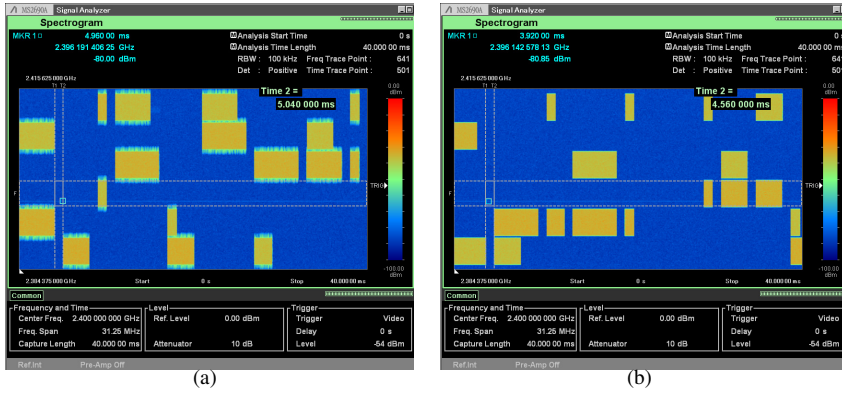
Figure 5.4: Comparison of the McF-TDMA scheme with and without filtering. (a) FPGA based filters disabled. (b) The 128 order FPGA based filters enabled.
