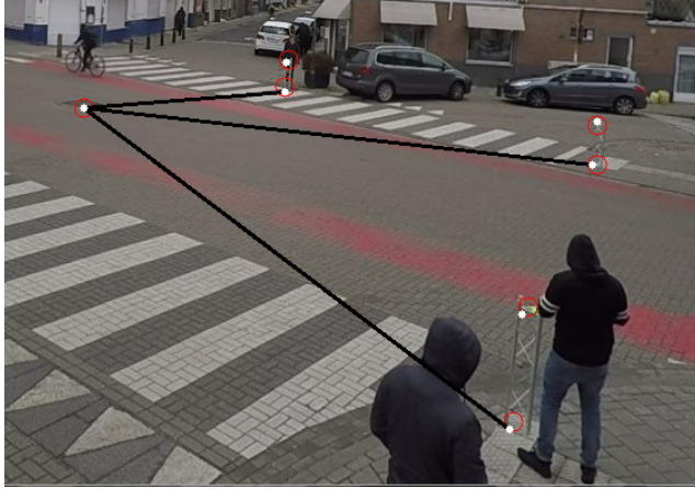
Figure 2.7: Example of the POSIT algorithm on the traffic intersection dataset of Ghent. The centres of the red circles correspond with the annotated positions. The white circles indicate the position of these points using the estimated camera parameters. Ideally, the centres of both circles are the same.
