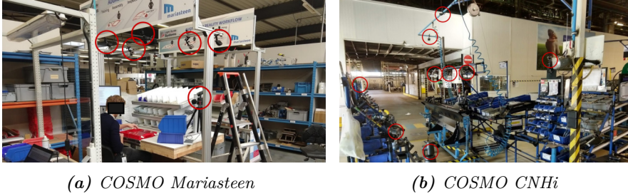
Figure 2.8: Different multi-camera setups from two use cases in this work related to the COSMO project. Cameras are indicated with circles on the overview pictures.
