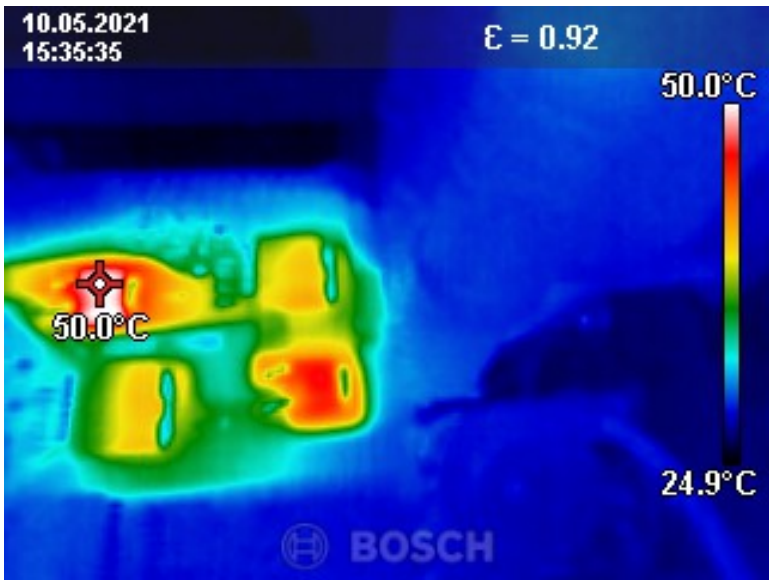
Figure 6.43: The temperature distribution over one asymmetric H-bridge module at 200 V DC-link voltage, 20 kHz switching frequency, 25°C water inlet temperature and 10 litre/min water flow rate.
