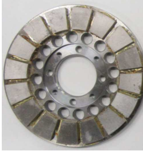
Figure 6.2: The rotor disk with the aluminium pieces instead of the magnets used in the experimental measurements.
