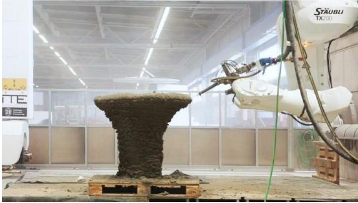
Figure 2.8 Example of spray-based 3D concrete printing, taken from [113].
