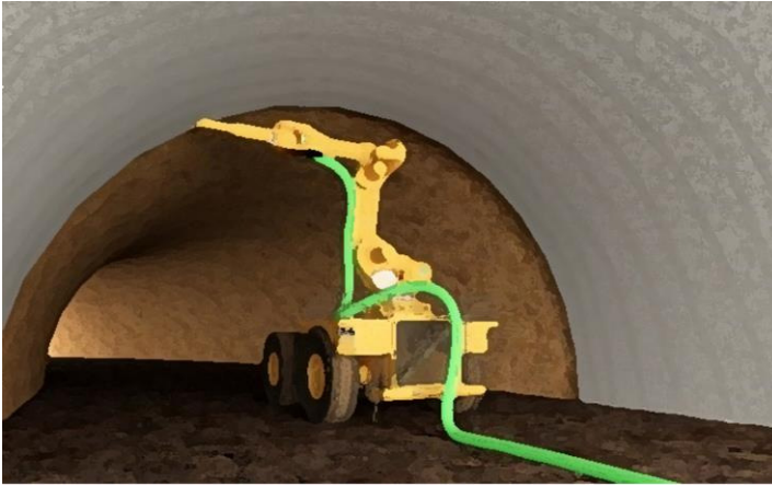
Figure 1.4 Schematic view of extending 3D concrete printing to hard rock tunnel linings.
