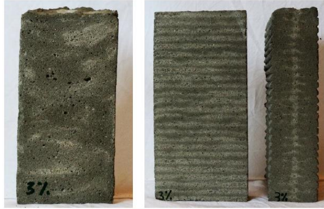
Figure 2.14 Insufficient mixing homogeneity, taken from [63].
