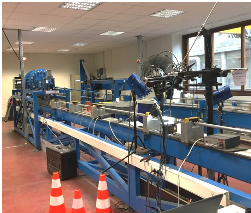
Figure 3.5. The split Hopkinson bar facility at Ghent University
