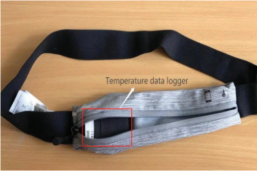
Figure 3. 4 Adjustable chest band with the temperature data logger (HOBO U12-012) inside.
