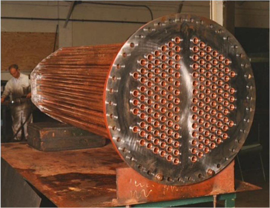
Figure 1-1: Copper heat exchanger used for example in offshore, pharmaceutical or petrochemical processes
