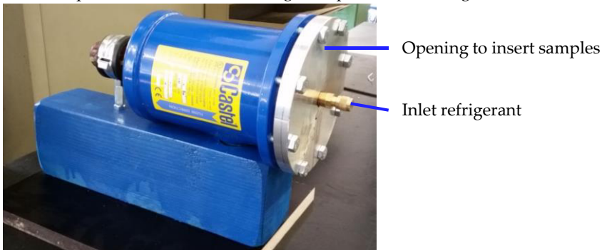
Figure 2-10: Pressure vessel to condition test samples for mechanical testing
