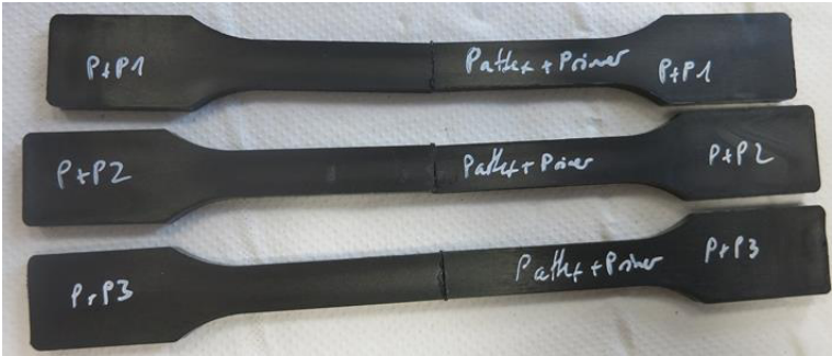
Figure 3-21: Dogbone samples which have been cut and re-joined using a glue connection to test the tensile strength of the connection
