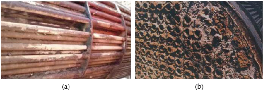
Figure 1-3: Reduction of efficiency and life-expectancy of a heat exchanger due to (a) corrosion and (b) fouling
