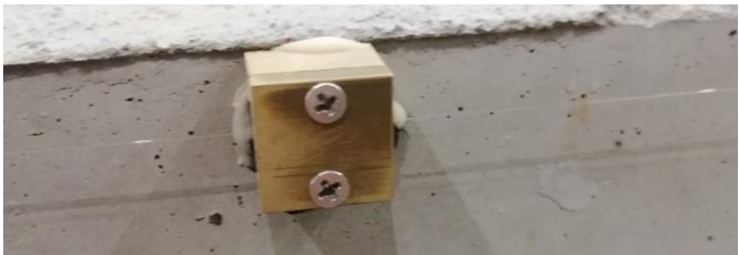
Figure VII-10: Optical fibre connected to the beam with clamping system
