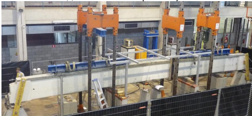
(b) Actual test set-up secondary beam
