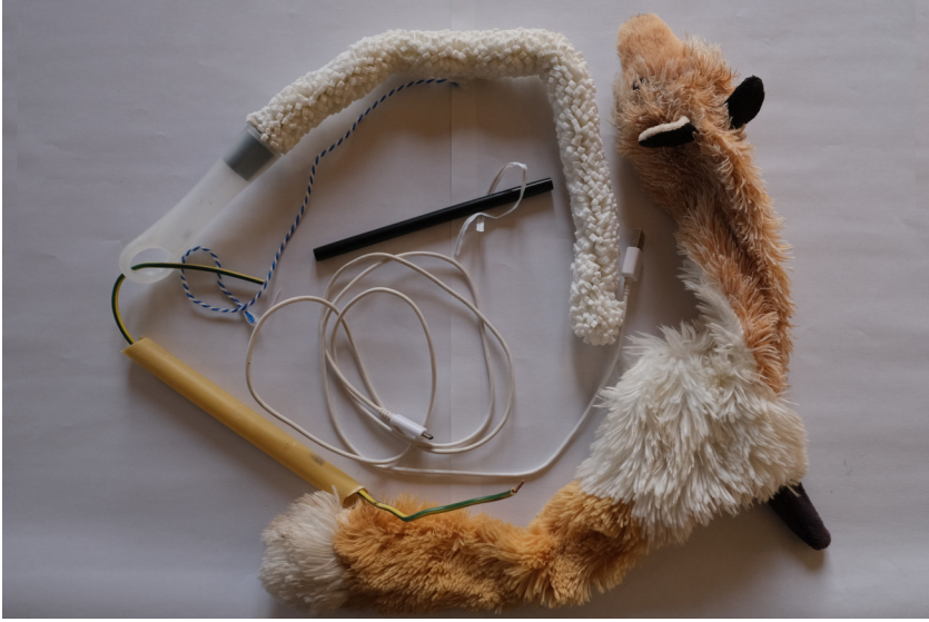
Figure 2.3 Examples of deformable linear objects and an application of putting an electrical wire into a rigid pipe.
