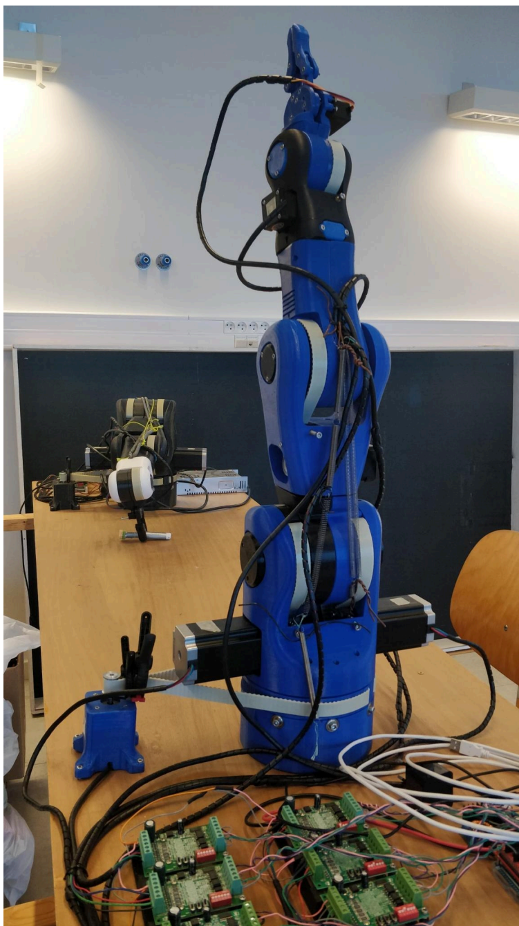
Figure 4.1 Picture of the constructed Moveo arm.
