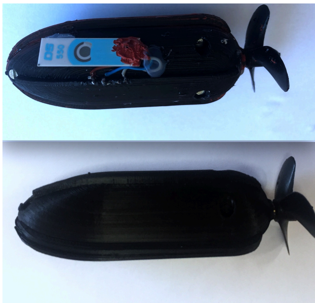
Figure 6.21: Impedance sensor Dropsens 550 attached to the hull of the submersible and connected to the internal microcontroller
