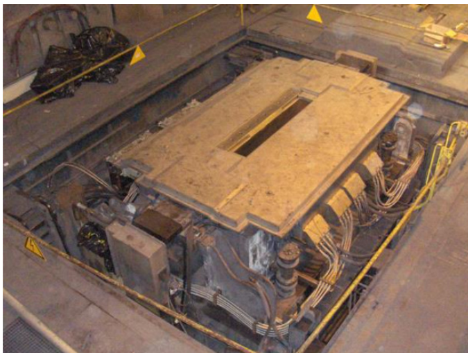
Figure 7.7: Snapshot of the EMS unit installed in ArcelorMittal Gent
