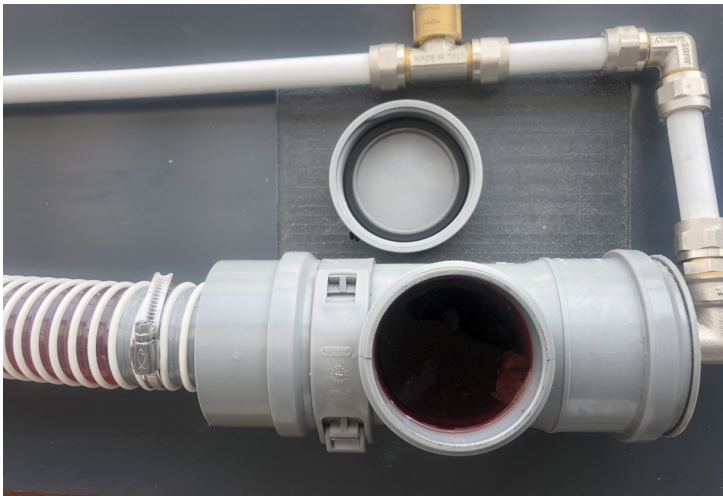
Figure 6.3: Snapshot of the extraction point in the lumped circulatory system
