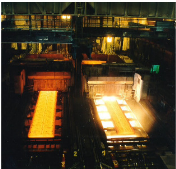
(a) View of the CC unit featuring cross cutters placed at the end of the casting line.
