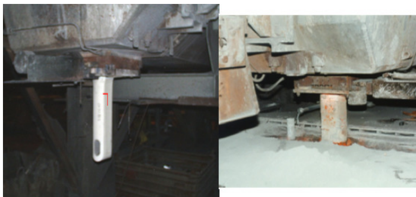
Figure 7.3: An illustrative example of a SEN ready for immersion (left) and a SEN in the mould (right). Observe the noisy environment and emerging deposits.
