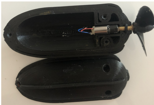
Figure 6.7: View inside the open submersible, hull, motor and propeller.
