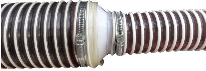
Figure 6.4: Snapshot of the transition area between the two flexible tubes of different diameter
