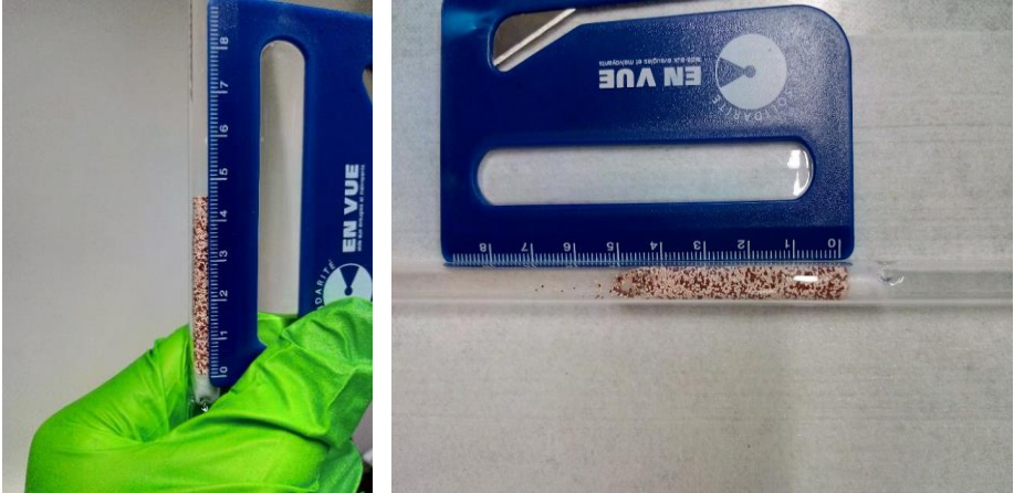
Figure C21: Photos of the reactor containing the solids used for the experiments. The red particles are those of the OC and the white particles are either the CC or the solid diluent, \alpha\text{-Al}_2\text{O}_3 . The ruler has a cm based scale.
