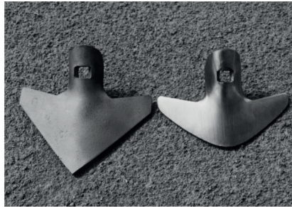
Figure 2-1 155 mm wide AS 1594 cultivator shares in new condition (left) and in worn condition after 9 km operation in abrasive South Australian soil (right) [63]
