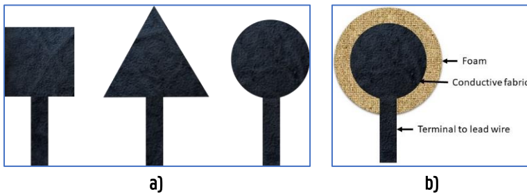
Figure 5.5: EEG textrode design: a) square, triangular, and circular active component of the textrode; b) schematic illustration of the EEG textrode on a foam
