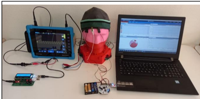
Figure 6.5: The photographic image of the EEG measurement setup
