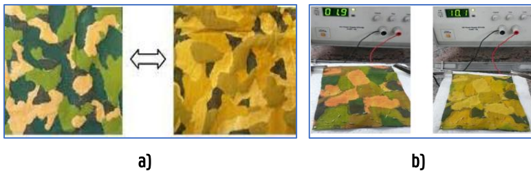
Figure 2.29: A thermochromic camouflage military fabric color change: a) heating to 60 °C; b) increasing voltage from 2V and 10V [30].
