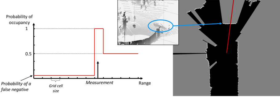
Figure 3.7: Example of a 1-D lidar sensor model (left) and the computed probability of occupancy map (right; brighter is more probable). The red line overlaid in the occupancy map shows the 1-D occupancy model applied to a slice of the lidar scan from the car (blue ellipse).
