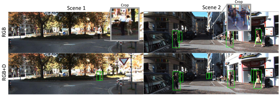
Figure 4.9: Examples of increased detection performance of the proposed early fusion ACF detector working on RGB and Depth images.
